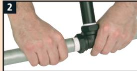
2. Screw pipe into fitting.
