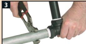
3. Do not over tighten. The right way to assemble a Threaded Pipe Fitting is finger tight plus one to two turns - no more!
