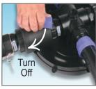
Step 2. Proceed to turn all the Pod Sprinkler Lines Valves off at the Pod Hydrants.
