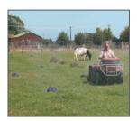
Step 5. Connect the Pod Sprinkler Lines to the ATV via the Hansen™ Tow System; proceed to drag the Pod Sprinkler Lines to the new location.
