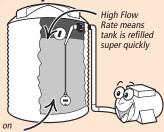
Pump only switches on when the tank is low
