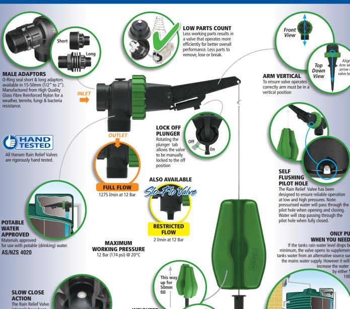
internals have been designed with a built in delay in closing, this helps to minimise water hammer. Note the Rain Relief Valve arm may be in the closed position but the valve may take up to 8 seconds to fully close. Do not force arm closed.
