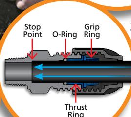
3. Insert the pipe into the fitting through the Nut, Grip Ring & Thrust Ring until it meets resistance at the O-Ring. Give the pipe a firm push past the O-Ring all the way until it hits the final stop point.
