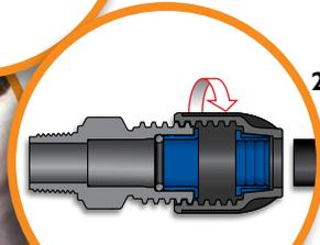
2. Undo the nut to the last thread, do not remove nut from the body.
