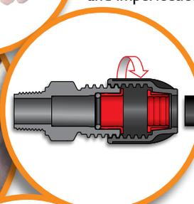
2. Undo the nut to the last thread, do not remove nut from the body.
