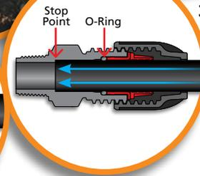
3. Insert the pipe into the fitting through the Nut and various internal components until it meets resistance at the O-Ring. Give the pipe a firm push past the O-Ring all the way until it hits the final stop point.
