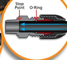
3. Insert the pipe into the fitting through the Nut and various internal components until it meets resistance at the O-Ring. Give the pipe a firm push past the O-Ring all the way until it hits the final stop point.
